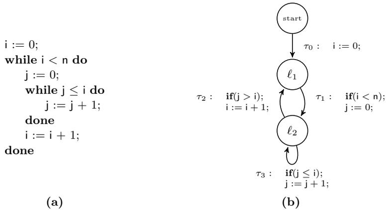
■ **Figure 1** Textual and control-flow graph representation of skeleton bubble sort routine
