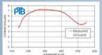
Obtained ratio of reflectance of a 45 nm thick amorphous Si thin film on quartz vs. wavelength.
